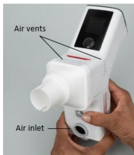
Figure 8: Air inlet and vents; these must be unobstructed while performing a test
