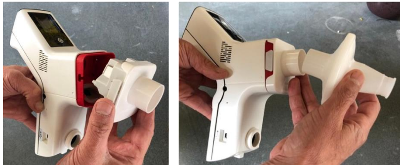
Figure 5: Click the valve house into place in the device and mount the Bacterial Viral (BV) filter onto the valve house.
