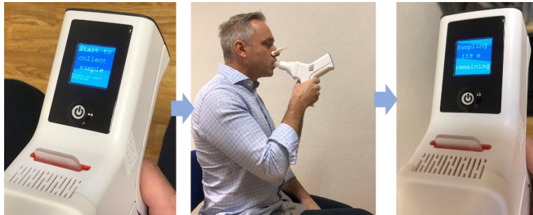
Figure 7: Ask test subject to pick up the device, inhale fully, and start breathing normally through the mouthpiece. The device beeps after 180 seconds timeout or when the sample fill detected.
